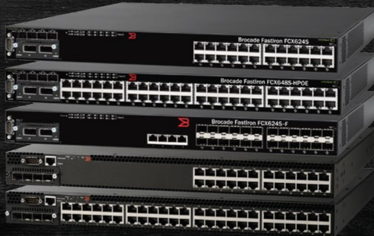
A switch is more intelligent than an **Ethernet hub**, which simply retransmits packets out of every port of the hub except the port on which the packet was received, unable to distinguish different recipients, and achieving an overall lower network efficiency.
